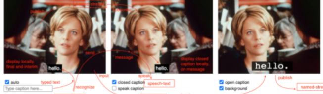
(c) Real-time open and closed caption in live published video using video-mix and speech-text
