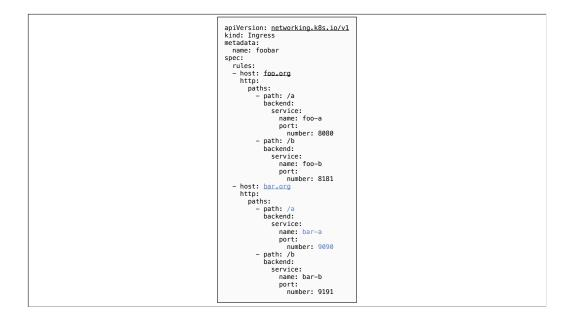
The third rule matches an HTTP request with a host header offer.org and a path of /a to proxy to a Pod that matches a Service named bar-a on port 9090
