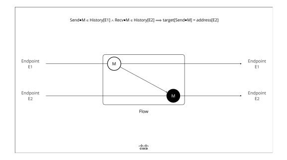
A pair or tuple of corresponding Send and Receive Events is called a Flow
