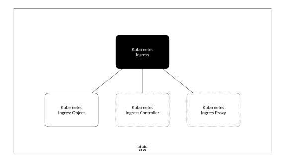
Kubernetes Ingress is indeed exceptional. For core abstractions, Kubernetes provides the resource and the controller out of the box. However, for Kubernetes Ingress, Kubernetes provides only the resource. The cluster operator must choose and instal the ingress controller and ingress proxy of their choice.
