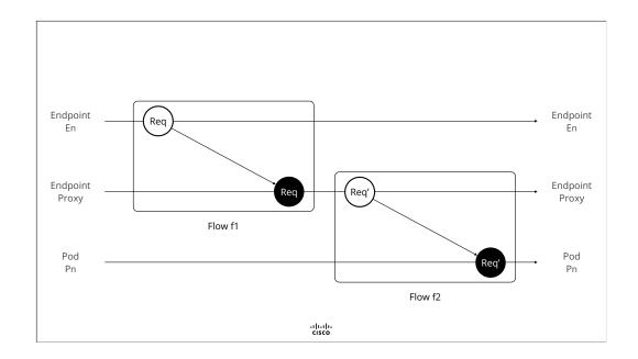
Represented as a Time Space Diagram. When the Kubernetes Ingress Proxy receives a request, it matches the request against the decision table and forwards the request so that a pod that matches the target service receives the request.
