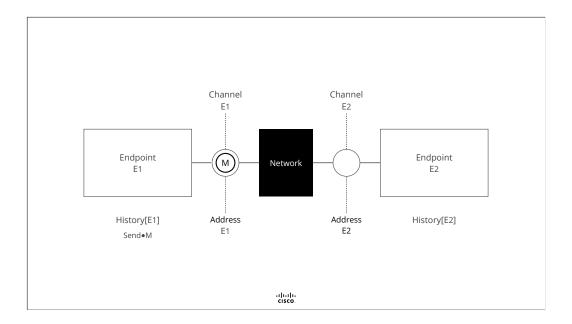
An Endpoint placing a message in its channel is represented by a Sent Event
