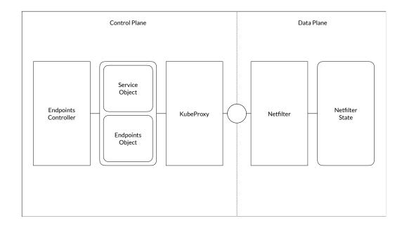
Similarly the Kubernetes Endpoints Controller is a core controller, it interacts exclusively with the api server. The Endpoints controller reads Service Objects and Pod objects and writes Endpoints Objects
