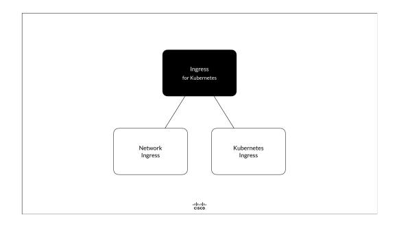
To enable the external consumption of a set of Kubernetes HTTP Services hosted on one Cluster via one HTTP Endpoint, Ingress for Kubernetes addresses two different concerns, Network Ingress as well as Kubernetes Ingress
