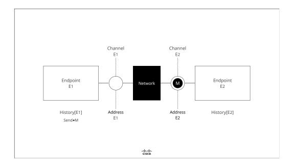
The network picks up the message from the sending Endpoint's channel and determines the receiving Endpoint's channel and places the message in that channel
