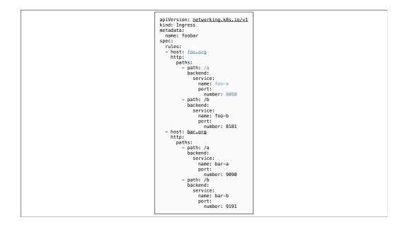
For example, the first rule matches an HTTP request with a host header of <u>foo.org</u> and a path of /a to proxy to a Pod that matches a Service named foo-a on port 8080
