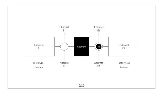
The Network placing a message in and endpoint's channel is represented by a Recv Event
