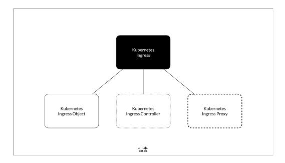
the ingress proxy accepts the request, match the request against the decision table specified by the ingress object and installed by the ingress controller and forward the request so that a pod that matches the target service receives the request
