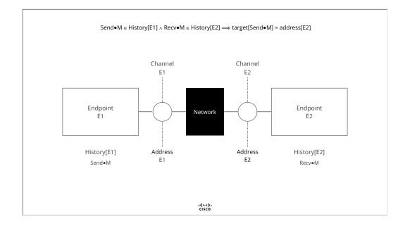
In this network model, Send Events are tagged with a target address. the network places the message in the channel of the endpoint who's address matches the message's target address
