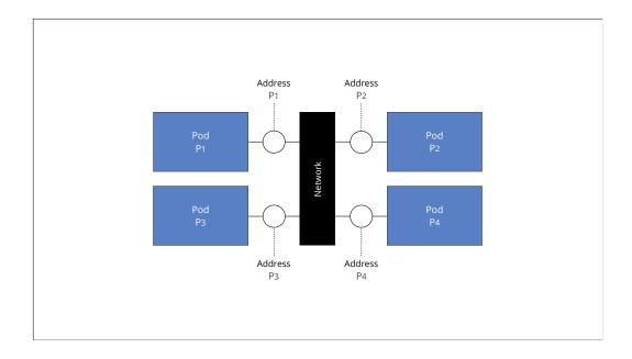
Network addressable endpoints are Pods. The Kubernetes Network Model specifies, that any Pod can communicate with all Pods without Network Address Translation
