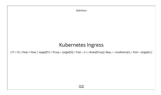
So in conclusion, Kubernetes Ingress can be defined as the set of all flow pairs, so that the first flow terminates at the proxy, the second flow terminates at a pod and there exists a rule in the decision table, so that the request of the first flow matches the conditions of the rule and the pod matches the target service of the rule
