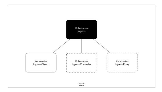
The ingress controller reads ingress objects and instructs the ingress proxy to create routing rules according to the decision table specified in the ingress object
