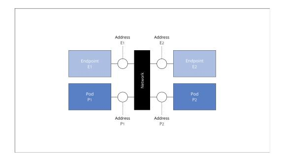
The Kubernetes Network Model does not specify weather external endpoints can or cannot communicate with Pods. As a consequence, depending on your closer, Network Ingress may be trivial or complex to implement
