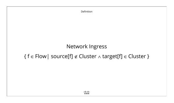
So in conclusion, Network Ingress can be defined as the set of all flows, that originate outside the cluster and terminate inside the cluster
