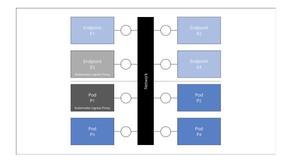
But either way, the task of the ingress proxy is to accept the request, match the request against the decision table specified by the ingress object and installed by the ingress controller and forward the request so that a pod that matches the target service receives the request
