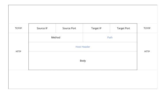
... and Host Header against its routing rules to determine the target Kubernetes Service to proxy the request to
