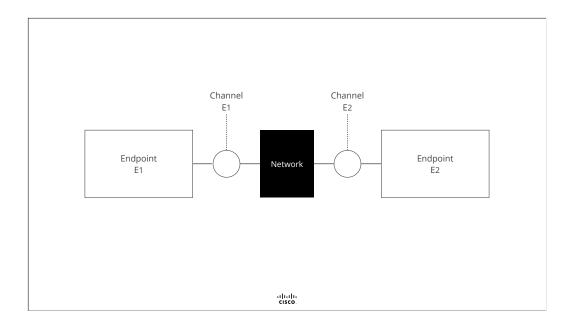
An Endpoint is connected to the network via a channel
