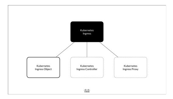
In effect, the Kubernetes Ingress Object defines a collection of HTTP request-level routing rules that determine the target of that request.
