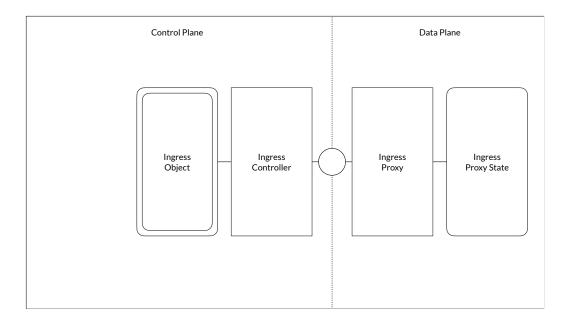
Now onto the ingress controller: an ingress controller is an edge controller, it interacts with the api server and with an ingress proxy. The ingress controller reads ingress objects and instructs the ingress proxy to create routing rules according to the decision table specified in the ingress object
