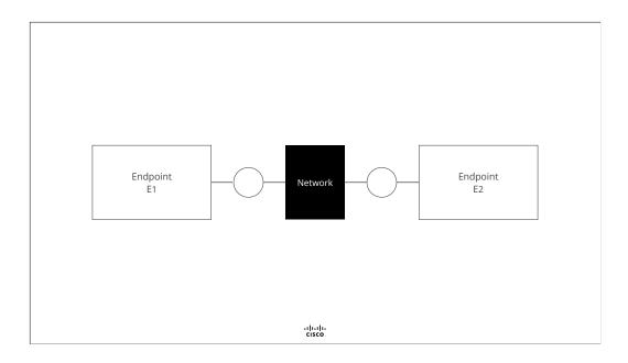
In software engineering, a distributed system is an unbounded set of components, from heron out called Endpoints. Endpoints communicate by exchanging messages via a **network**.
