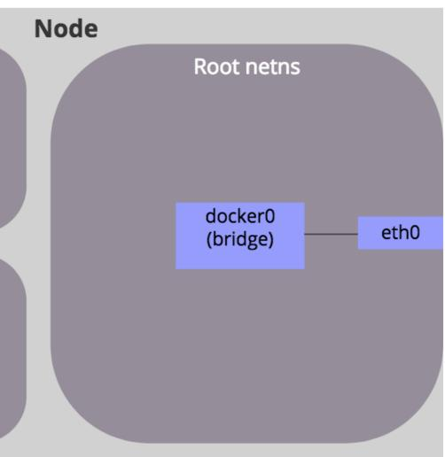
Docker creates a VETH pair (virtual ethernet device). This is like two network devices with a pipe between them. It attaches one of the devices to the docker0 bridge and the other it moves into the container's network namespace and names it eth0 within that namespace.
