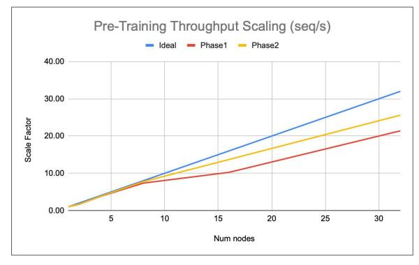
BERT Phase 1: batch\_size\_per\_gpu = 64, seq length = 128 Phase 2: batch\_size\_per\_gpu = 16, seq length = 512
