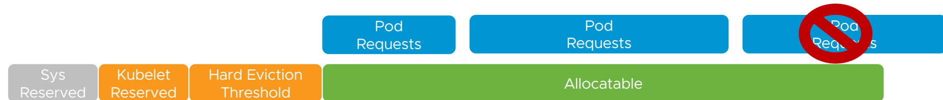
Scheduling of Pods with Requests and “Node Allocatable”
