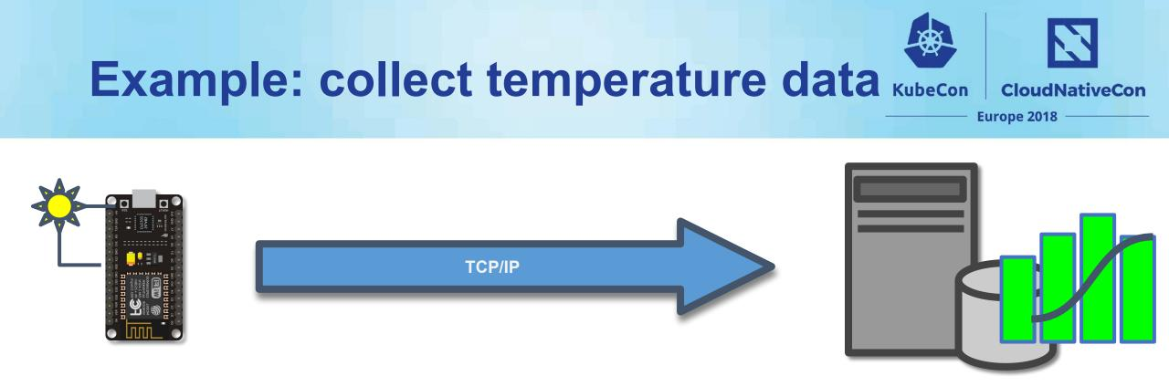
Collect temperature data from microcontroller Use protocol buffers to serialize data on device Send data over TCP/IP to remote server Post data to time series database for visualization
