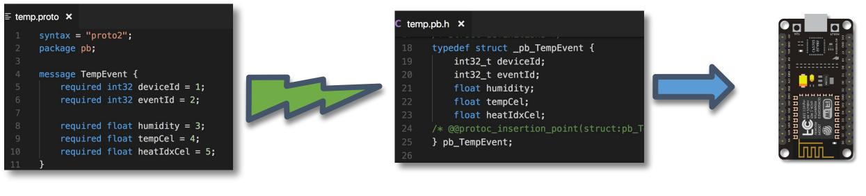
$1_{\text{Define IDL}} \quad 2_{\text{protoc}} \quad 3_{\text{Integrate C code}}$
