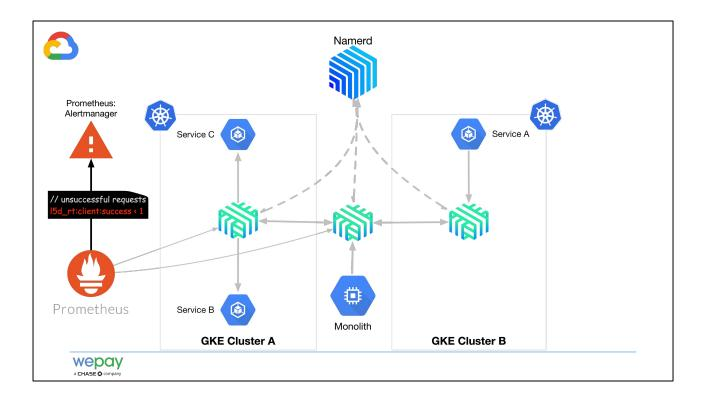
Aggregated metrics are used for **alerting on important events** in the environment.
