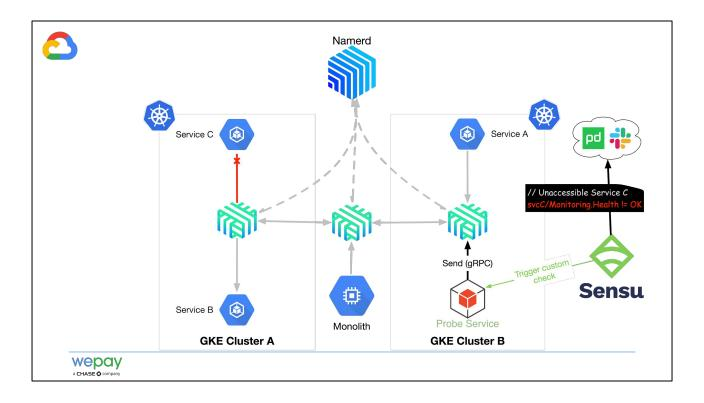
Custom checks trigger alerts based on their own thresholds and alerting criteria.
