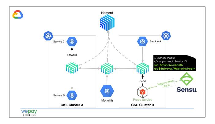
**<u>Challenge</u>**: Checking that all expected services are routable within the scope of service mesh in the environment.
