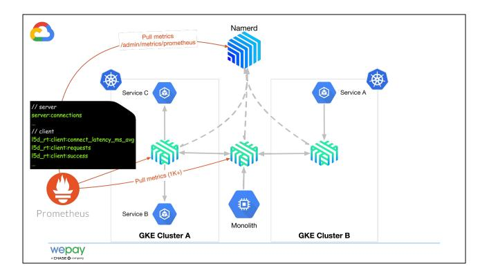
Linkerd and Namerd instances generate over 1K metric points related to server and client that is gathered by Prometheus for visualization and debugging.
