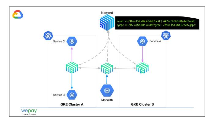
Since we have **both K8s and non-K8s services** in the environment, using **Linkerd 1** to provide service mesh inside and outside of K8s with the **same discovery scope** within a single environment.
