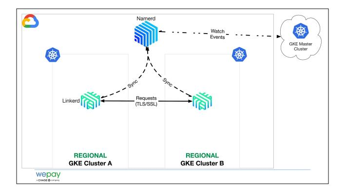
Service mesh generally involves a data and a control plane, Linkerd proxies and Namerd, respectively:
