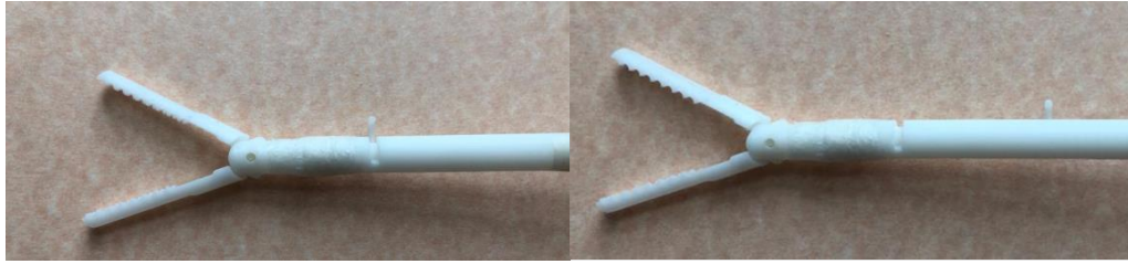
Figure 31: Extruding and sliding the hook feature of 2 nd prototype
