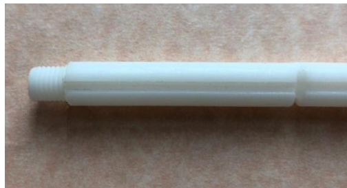
Figure 28: Zoom in of the screwing feature at the connecting region between the body and the handle of 2 nd prototype
