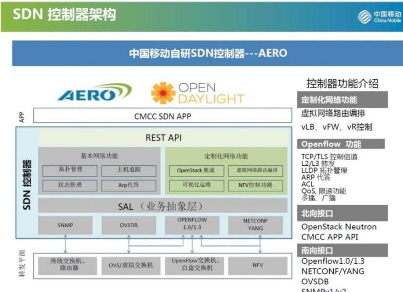
AERO: SDN controller developed by China Mobile based on OpenDayLight
