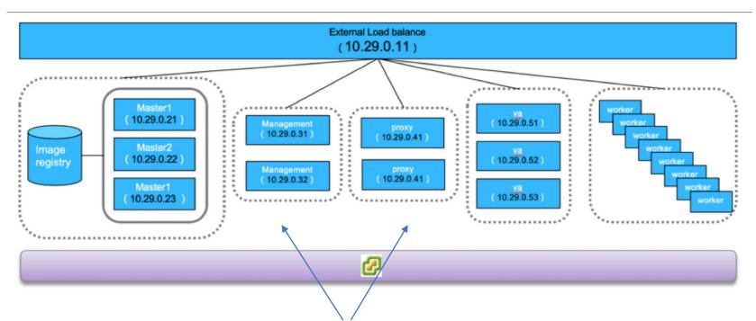
The istio control panel is running in management and proxy nodes.
