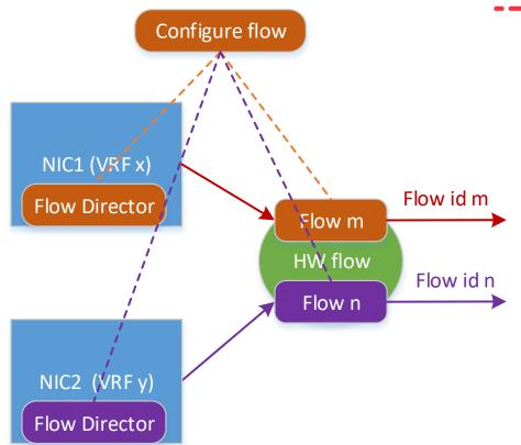
If having same 5-tuple packet matching on 2 different VLANs or even on 2 different interfaces, they should be treated as different flows.
