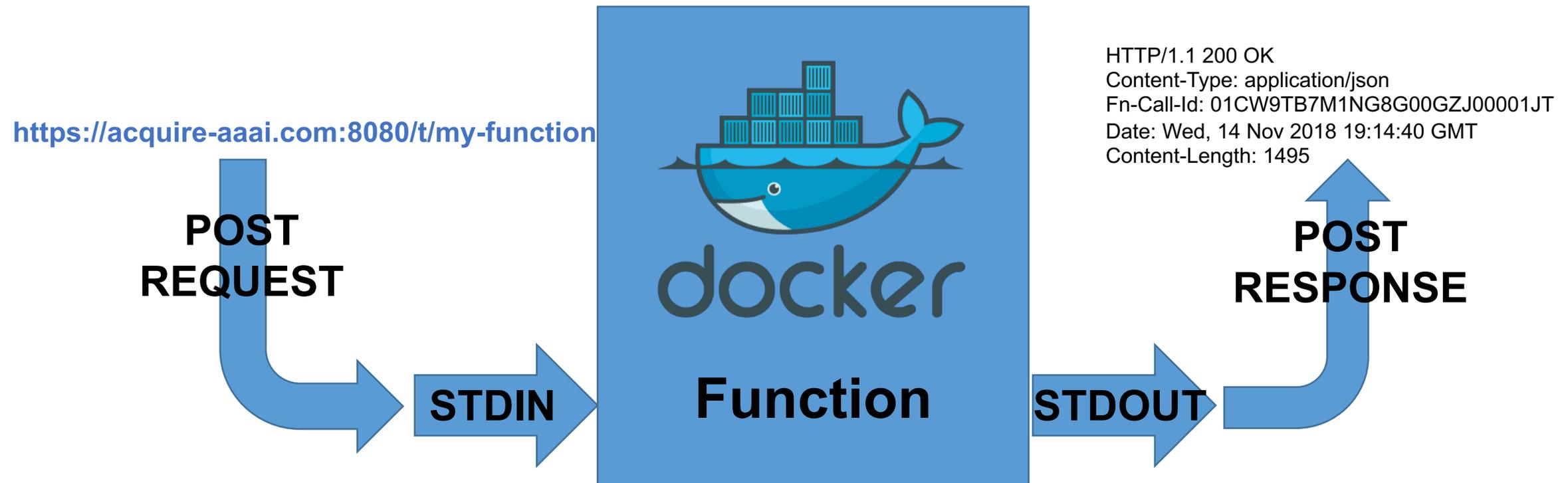
Code to run the function is wrapped into a docker container. This is allocated to hardware in response to a trigger (e.g. https). Input data is encoded via POST and piped in as STDIN to the container. This is processed by the function, with resulting STDOUT returned as a HTTP response
