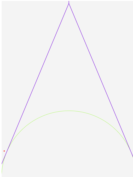
FIGURE 3.10: An AWP Voronoi diagram of three sites, one site with a large weight and its corresponding circle and two sites that lie lower than the top of that circle
