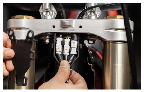
*Step 2: Connecting the Electronic Clutch Disconnect the throttle connector.*
