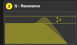
Like the original MS20, Sallen-Key offer a non-linear feedback path. This design avoid the filter to clipping when self-oscillating, but also give it is unique color. input gain. You can attenuate the input gain with the dedicate attenuator.
