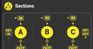
GOMA can be use as a flexible mixer with virtualy infinite channels. The modules is made of 3 identical sections. If nothing is plug into the output of a section the signal flow allowing to create infinite mixer.
