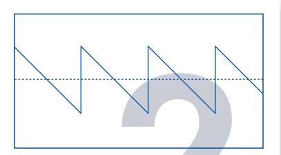
**INVERTER 1** Inverted copy of input 1
