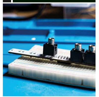
Input of bottom section (the 5th jack starting on top of the module) need to be install like on the picture. Make shure that switched leg is not bend or input 2 will not be normalised to inverted output of top section.
