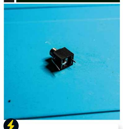
the middle leg of jack connector it's call « switched » it's handy to normalize input. In the case of Dual Rectifier only input 2 is normalised to the inverted output of top section.
