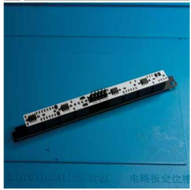
Return the module and make shure that each pins of each jack is place correctly. Look at each holes it should be a jack connector legs coming thru. If it missing one make shure to re-place correctly the connector before soldering.
